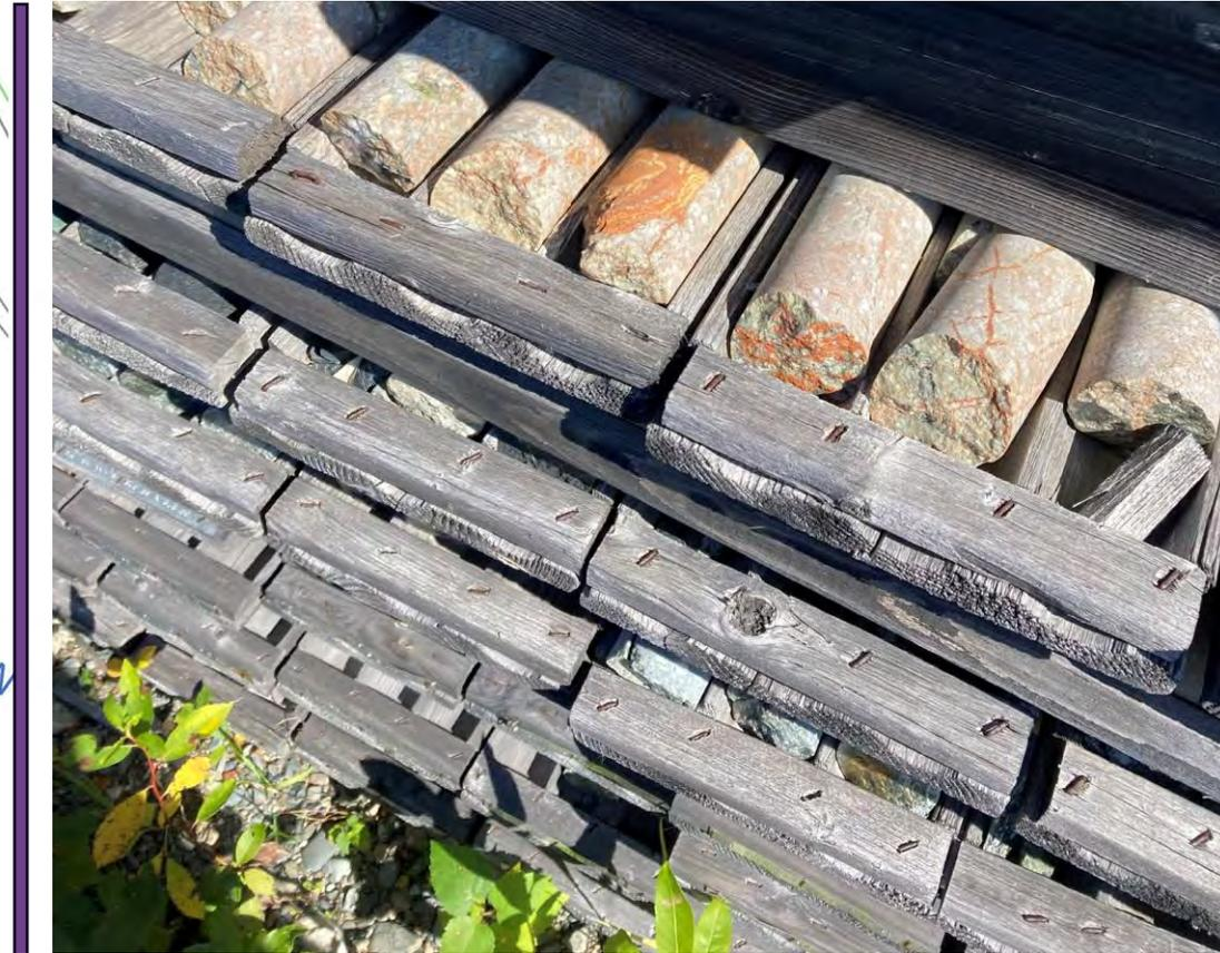
Historical Drill Holes (DDH) in Open Pit, showing lack of sufficient sampling for proper resource characterization
