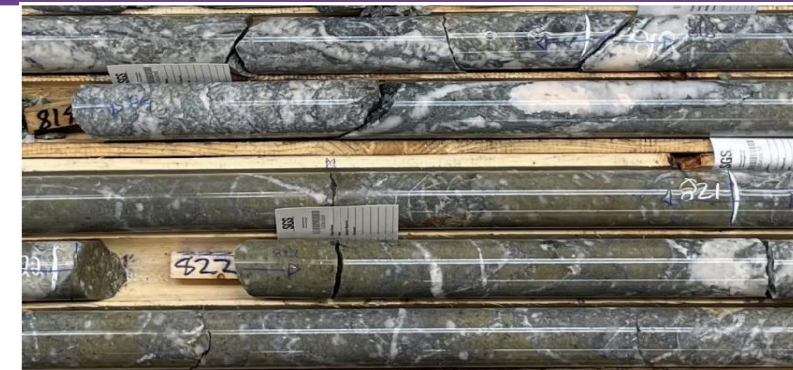
Representation of mineralized and altered porphyry core from DQ23-02 (25.0 m of 1.69 g/t Au) ; bottom of hole ended in mineralization and this zone is subsequently being extended by additional drilling. – core depth of 814 m
