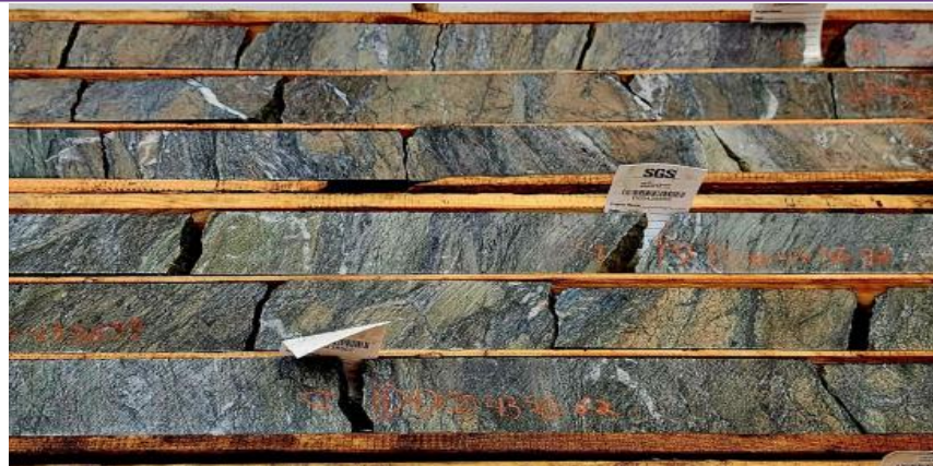
Representation of mineralized and altered core from DQ23-02 (10.65 m of 3.97g/t Au (includes 5.0 m of 5.34 g/t Au)) - core depth of 540.25 m
