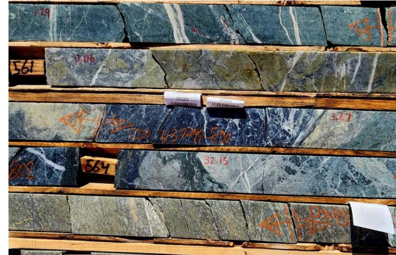
Representation of mineralized & altered core from DQ23-05 (10.8 m of 15.8 g/t Au (includes 3.4 m of 27.24 g/t Au)) – core depth of 563 m
