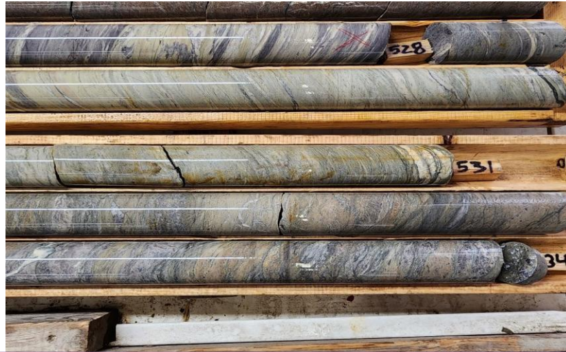
Representation of mineralized & altered core from DQ23-01 (11.7 m of 5.63 g/t Au) core depth of 531.3 m
