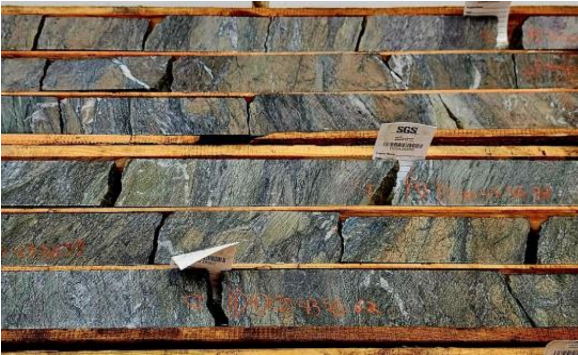
Representation of mineralized and altered core from DQ23-02 (10.65 m of 3.97g/t Au (includes 5.0 m of 5.34 g/t Au)) - core depth of 540.25 m
